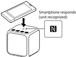
Follow the on-screen instructions to establish the connection. When the BLUETOOTH connection is established, the **Ⓜ** (BLUETOOTH) indicator on the unit stays lit. To disconnect, touch the unit with the smartphone again.
