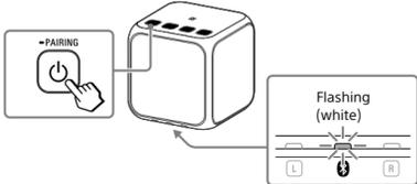
2 Press and hold the **⏻ (power) – PAIRING** button until beeps are heard and the **Ⓜ** (BLUETOOTH) indicator begins to flash quickly.
