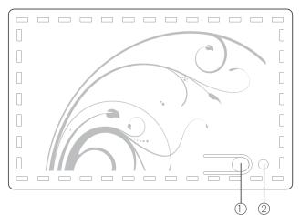
1. Timing button: Press this button once to show both input and output display resolution and while the OSD is still on the screen press it again to select output resolution from 1280x800, 1366x768, 1920x1200, 720p, 1080p 2. Power LED: This LED will illuminate when power is connected.
