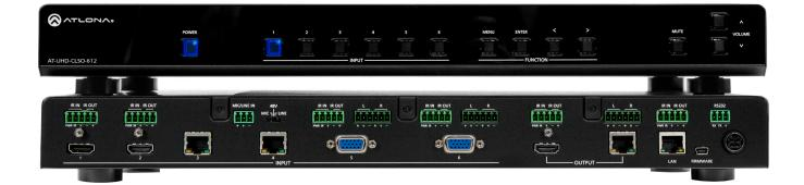
Easy to integrate, the CLSO-612 was designed for conference and classrooms with inputs at lecterns, tables, and desks. Sources and displays can be up to 230 feet (70 meters) from the switcher with HDBaseT inputs and outputs. Local HDMI and multifunction analog inputs work with any source. Combined with great features such as: 4K up/down scaling, microphone ducking, and audio control, this is the core component of your presentation AV system.
